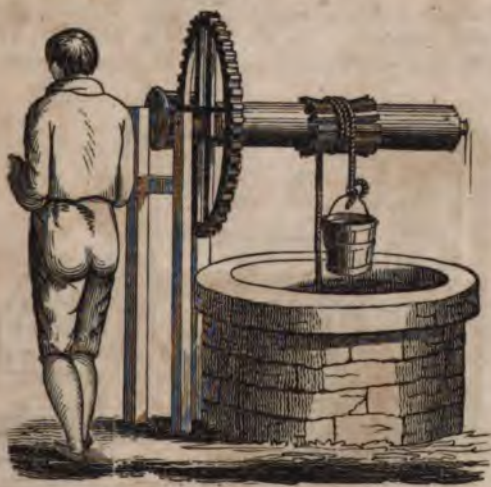
No. 21. Windlass with cog-wheel and pinion.
